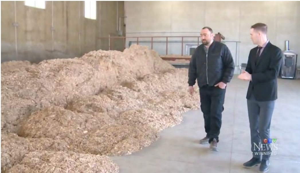
Figure 91: Wood chips on walking floor at Vermillion Hutterite Colony's biomass plant 113
