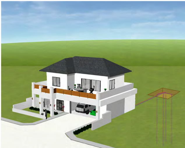
Figure 101: Schematic of vertical loop ground source heat pump system 141
